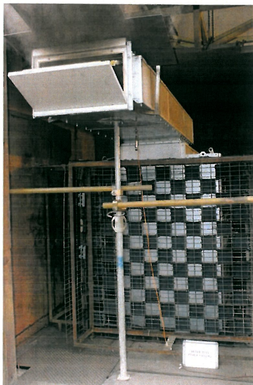
Photo No. 10 After test PEHLA 13032Ra / 03 Test object, side view with indicators and opened hatch at the end of the outlet
